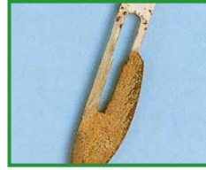
Rust formation on a scalpel blade. Cause: Not stainless steel as this is a disposable product.
