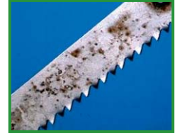
Rust formation on a chromium-plated saw blade made of carbon steel. Cause: Defects in chromium layer.
