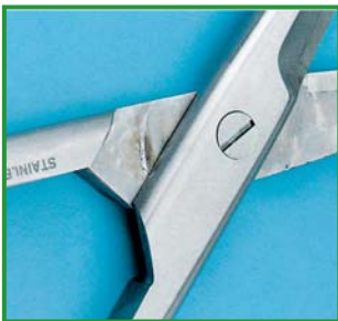
Fretting corrosion due to inadequate lubrication
