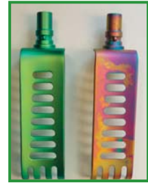
Left valve: brand new - uniformly green Right valve: machine-cleaned - strongly discolored
