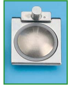
Leaky trocar flap valve due to gasket swelling as a result of oil contact.
