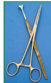
Contact corrosion through contact of stainless steel and brass
