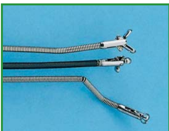
Biopsy forceps damaged by sheer force
