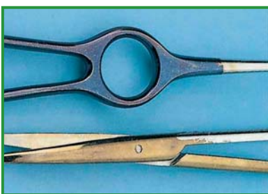
Instruments discoloured by silicic acid
