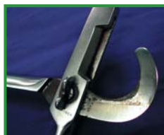
Chrome plate castrations forceps. Damage to chrome parts lead to corrosion films. Danger of transfer of rust onto stainless instruments.
