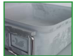
Discoloration by pickling on aluminum
