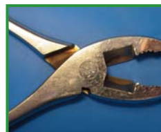
Chrome plate pliers from DIY store. Non-chrome parts (e.g. joint) lead to corrosion films. → Danger of transfer of rust onto stainless instruments.
