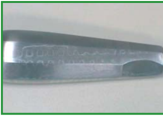
Carry-over of cleaning agent residues due to insufficient rinsing
