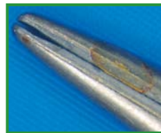
Acid attack on welds and hard metal inserts, with consequential damage in the form of extensive wear Cause: Overdispensing
