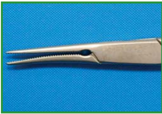
Deformation caused by improper handling
