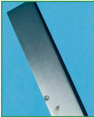
Corrosion on chisel
