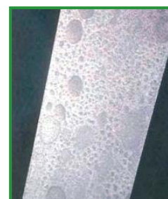
Instrument surface with drip-like discoloration
