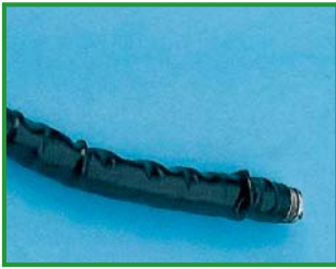
Swelling at distal end of fiberscope
