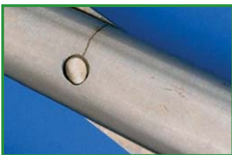
Hairline fracture adjacent to hinge on a pair of scissors
