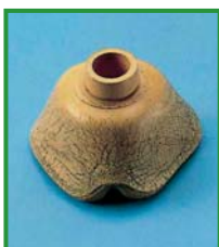
Cracks caused by ageing on breathing mask
