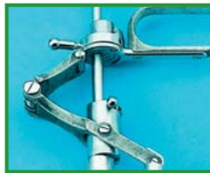
Damage to aluminium components only. Cause: use of highly alkaline detergent
