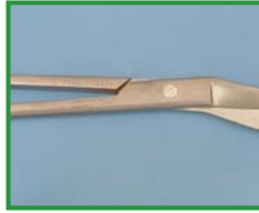
Stainless steel instrument with acid attack (brown tarnishing). Cause: Overdispensing.
