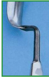
Surgical hook with shaft made of hardened Cr-steel showing black discoloration and handle that has remained bright and blade made of non-hardened CrNi steel
