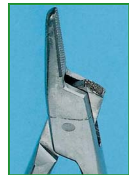
Jaw breakage on suture holder
