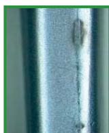
Contact corrosion between two instruments both made of stainless steel
