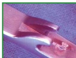
Suture holder with spring abrasion
