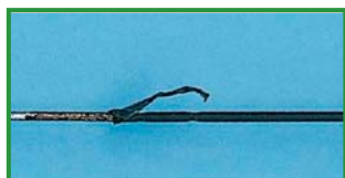
Damaged insulation on HF instrument
