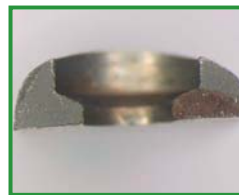
Breakage at countersunk screwhead
